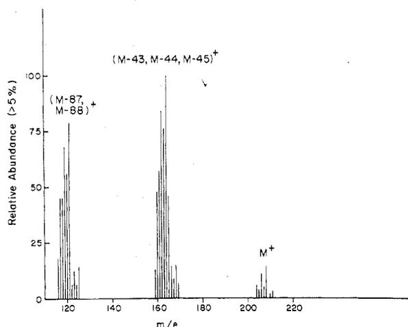
Figure 1. Mass spectrum of  $\text{Sn}[\text{N}(\text{CH}_3)_2]_2$  at 80 eV.
