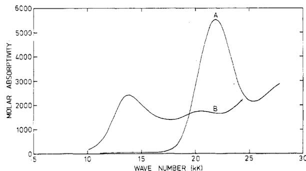
**Figure 6.** Calculated spectra of the models  $\text{Se}_4^{2+}$  (A) and  $\text{Se}_8^{2+}$  (B).  $\text{Se}_4^{2+}$  was calculated on basis of 10 measured spectra;  $\text{Se}_8^{2+}$  was calculated on basis of 14 measured spectra.
