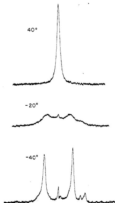
Figure 2.  $^1\text{H}$  NMR spectrum of  $\text{Sn}[\text{N}(\text{CH}_3)_2]_2$  at 60 MHz in *o*-dichlorobenzene at 40, –8, and –40°.
